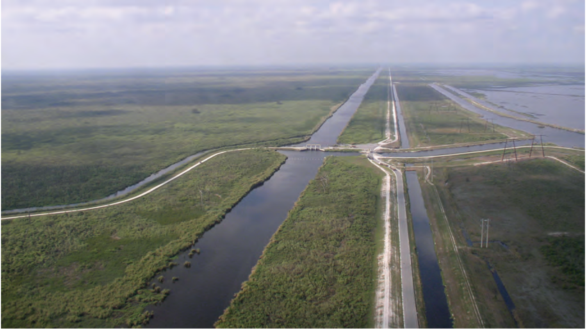
FIGURE 13.4 Enormous canals have altered the natural hydrology of the Everglades, and provided a conduit for nutrient enriched water to enter the wetlands.
