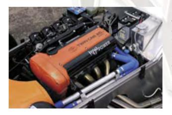
**4AGE 20v vvti** - This unit was the next generation 4age engine that was not installed in UK Toyota cars. It is a very high spec engine with side draft throttle bodies and variable valve timing as standard. This engine possesses all the advantages of the 16v but it is more refined and offers more power in standard form. We provide this engine with mapped ignition to facilitate ease of installation and improve after sales service.
